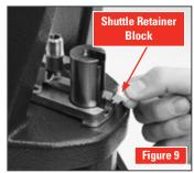
The primer shuttle should now slide out through the slot in the front of the ram (Figure 6). When finished changing punches, reverse the above steps to re-install the shuttle.
