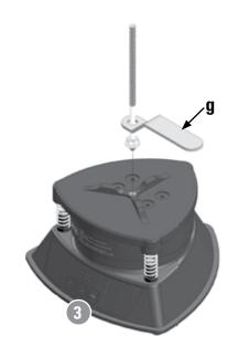
**6.** The Lid is held in place with the second Washer and Wing Nut.
