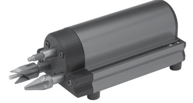
The Lock-N-Load<sup>®</sup> Case Prep Trio makes case preparation faster and easier than ever. Included are chamfer and deburr tools, with plenty of onboard storage for optional case prep accessories like our primer pocket cleaners, case neck brushes, and many other 8-32 threaded tools.
