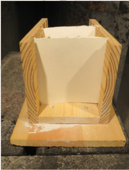
Witness card test fixture. Simple cardboard box can achieve similar results for a field-expedient test.
