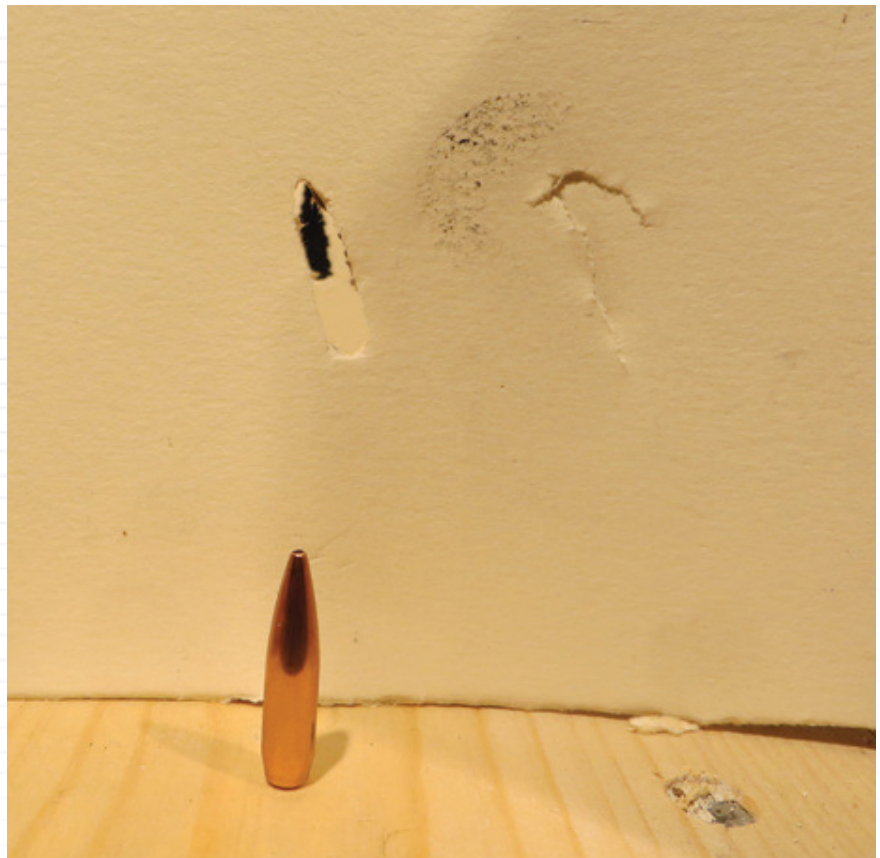
Results of witness card test. Bullet was traveling nearly sideways as it penetrated both first and second witness cards.
