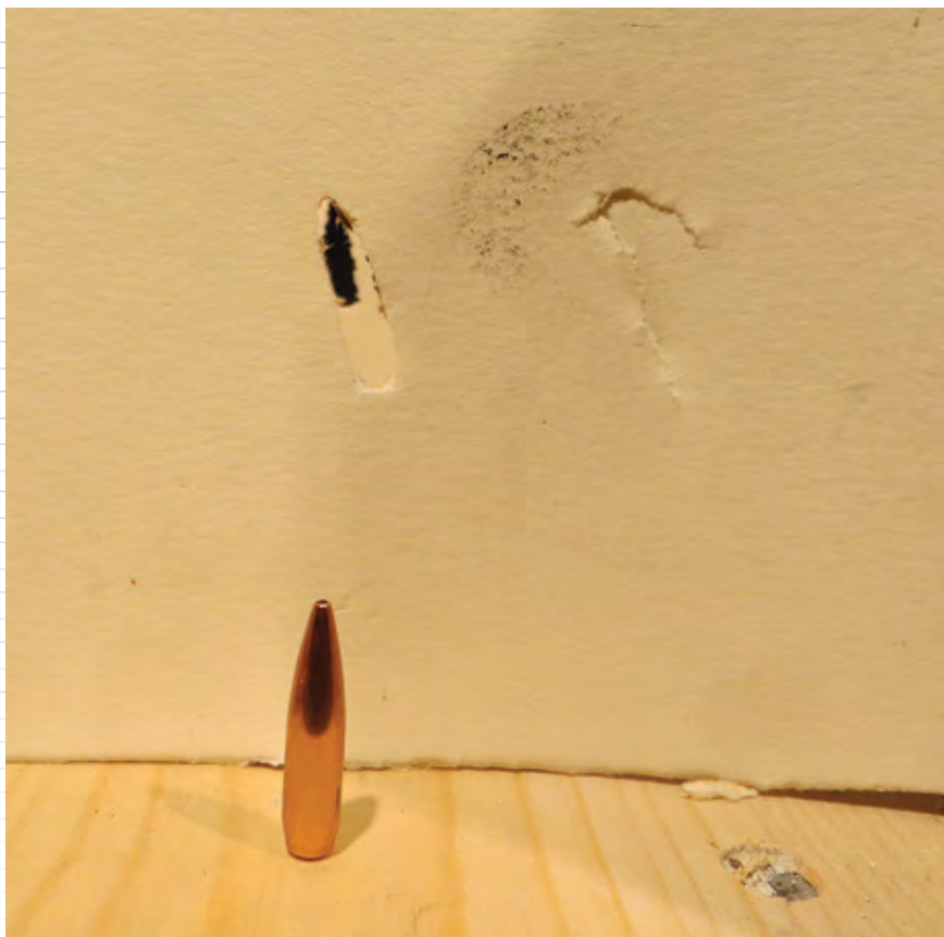
Results of witness card test. Bullet was traveling nearly sideways as it penetrated both first and second witness cards.
