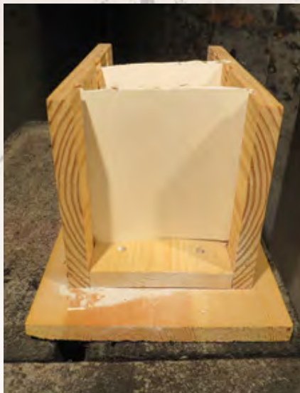
Witness card test fixture. Simple cardboard box can achieve similar results for a field-expedient test.
