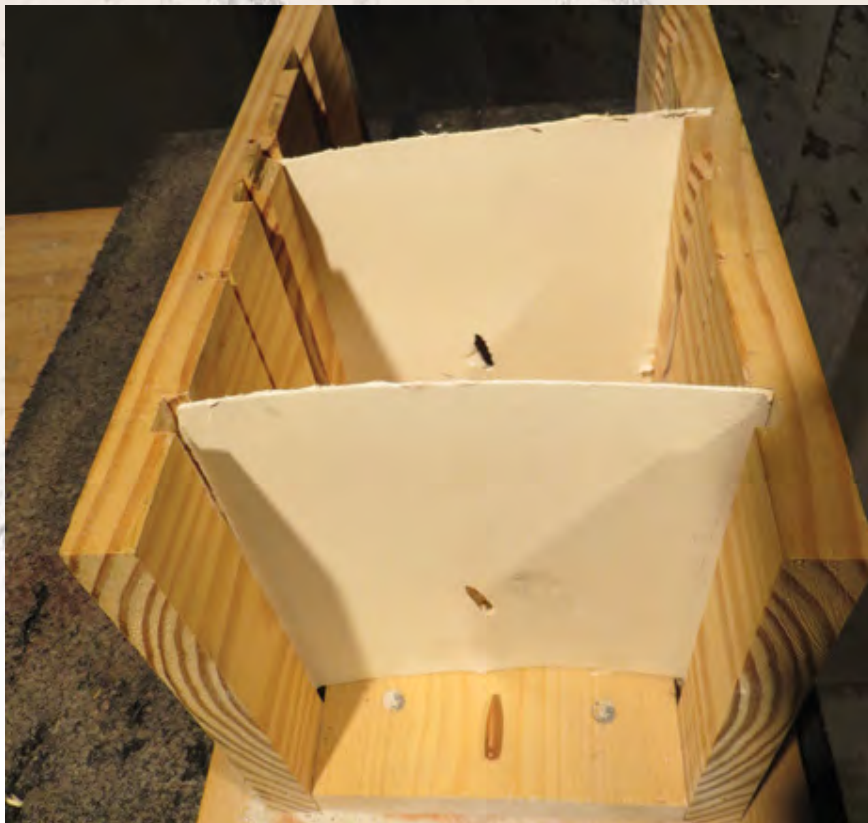
Bullet position changes from first card to second card as bullet tumbles.
