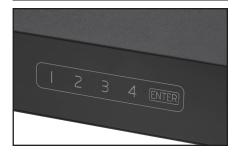
5. With the safe open, enter the new code followed by ENTER to confirm the safe is working properly. The motor should cycle after each correct entry.
