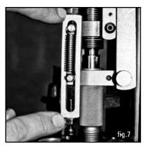
**Step 7:** To adjust for more case mouth flare, continue to screw in the bottom cap screw, for less case mouth flare, back it out. Make small adjustments.
