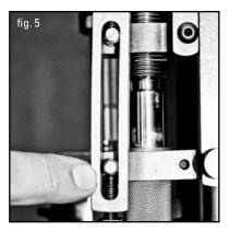
**Step 5:** Place an empty, primed case into the station of the shell plate that will rotate to the powder measure. Raise the ram which will cycle the powder measure to the top of its stroke. Thread the bottom cap screw in until the threaded end bottoms out on the lower hex spring mount (fig. 5).
