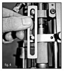
**Step 4:** Install the PTX<sup>™</sup> Powder Measure Stop over the hex spring mount with the cap screw that is protruding on the top (fig. 4).
