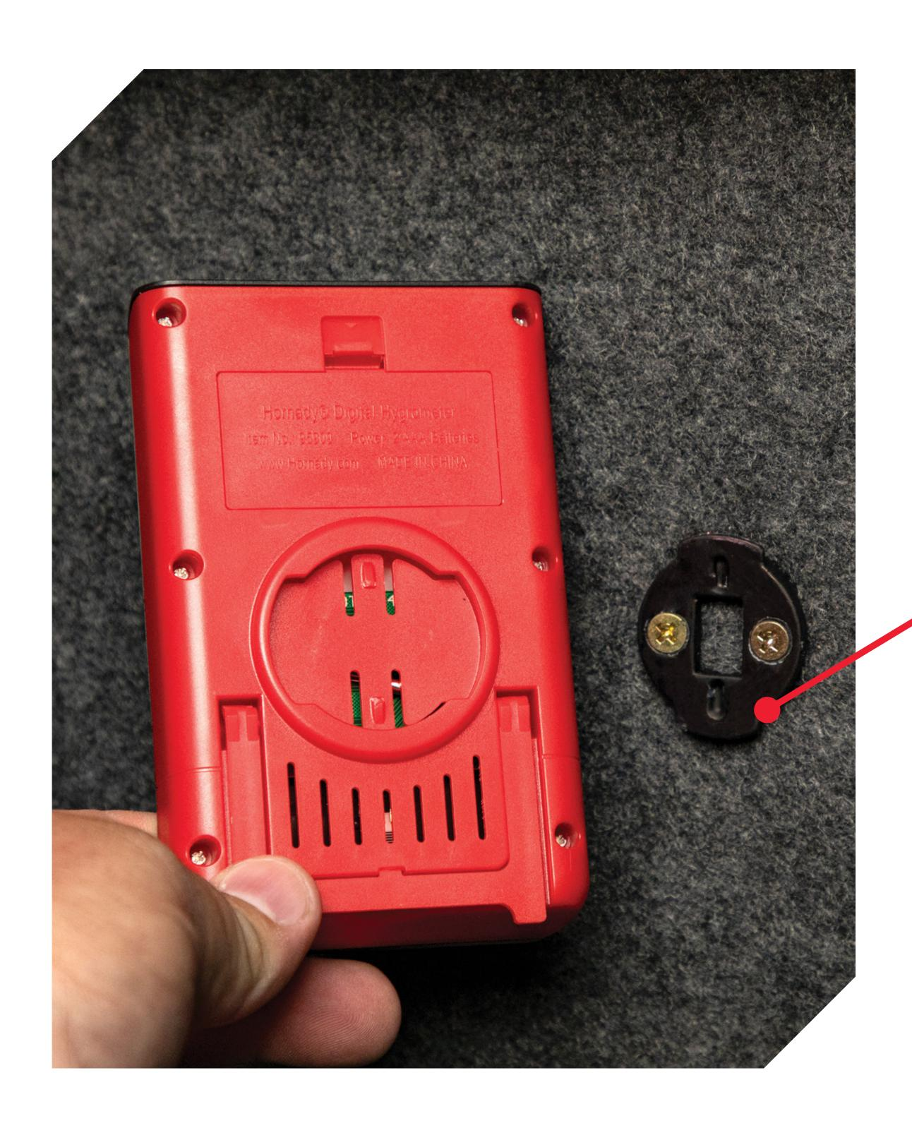
Installs on door or wall with quick-connect bracket
