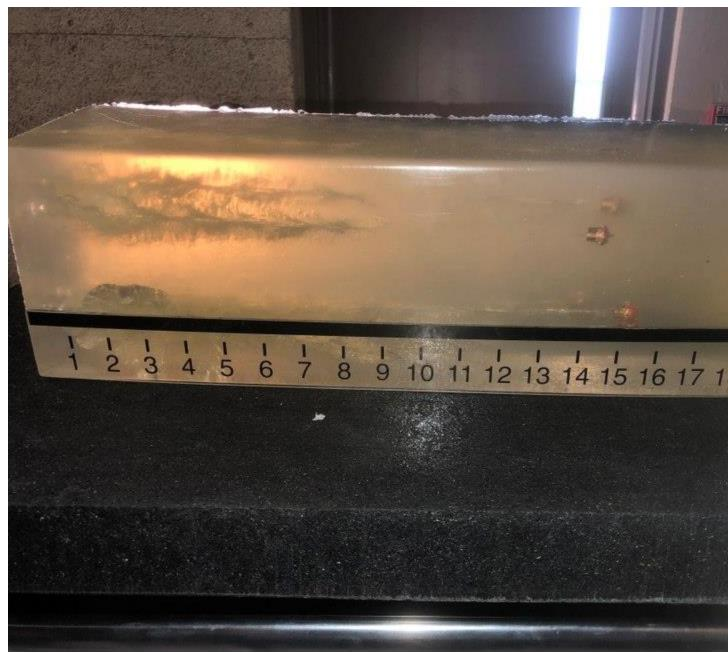
The 10% organic gelatin used in our tests delivered predictable results, with bullets expanding and penetrating as they had in previous efforts from many sources. Shown is the 9mm Hornady Critical Duty 135+P. (Photo/Mike Wood)
