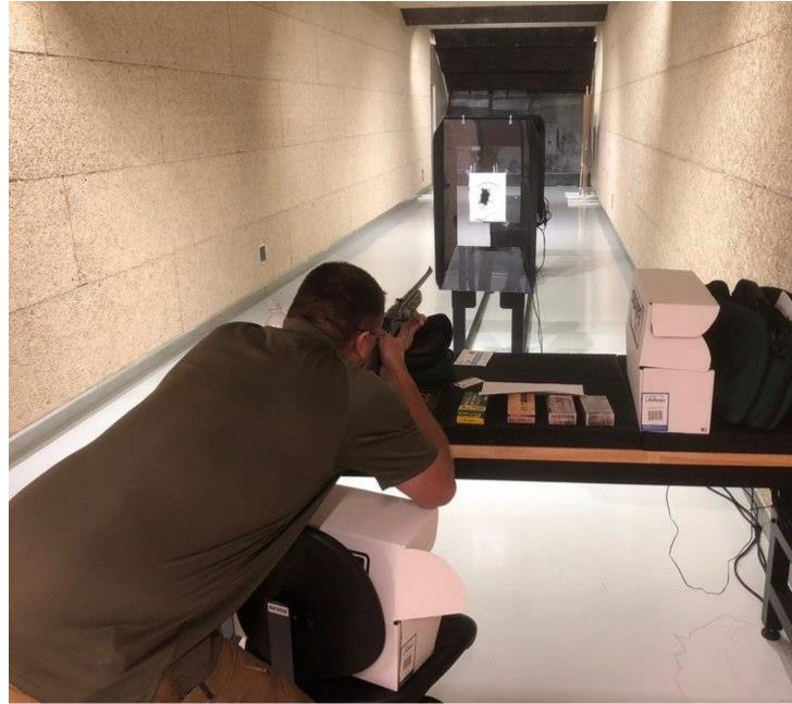
Chronographing the BB gun at the test facility, prior to firing calibration shots into the gel. (Photo/Mike Wood)
