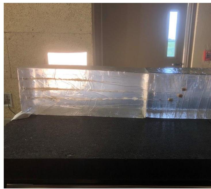
Sometimes, bullets would not stay inside a single block, and had to be recovered from a secondary block behind the first. (Photo/Mike Wood)
