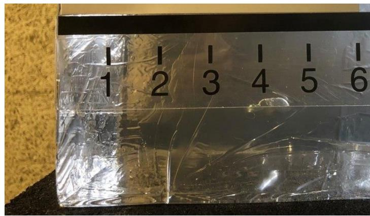
As seen here, the calibration BBs bounce back in the clear synthetic gelatin, just as they do in 10% organic gelatin. Unfortunately, the overall penetration of the BB in the clear synthetic exceeds FBI standards. (Photo/Mike Wood)
